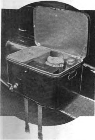
The ingeniously designed, compactly constructed refrigerator which is carried strapped to the left runningboard of the special Studebaker sedan illustrated above.
